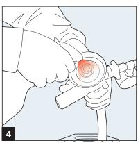
Sanitize KeyKeg filling head with disinfectant and fill line with beverage untill top.
