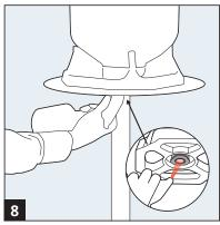
Sanitize inside valve with disinfectant and clean with warm water after filling, when still upside down.
