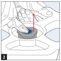
Remove the dust cap and discard. Do not replace the dustcap after filling!
