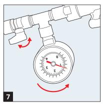
Keep counter pressure to a level well over the equilibrium pressure of the beverage and open gas valve gradually. When pressure is '0' leave the beverage valve open for an extra 3 seconds.
