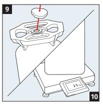
Place KeyKeg right-side-up. Weigh the KeyKeg and seal with a snap cap.
