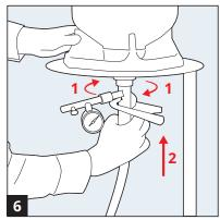
Connect the KeyKeg filling head and open the beverage valve.
